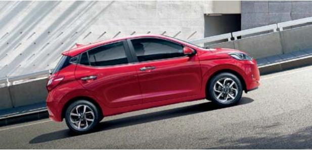
Hillstart assist control HAC maintains braking power after you have removed your foot from the pedal to prevent rollback and releases the brakes the moment your foot touches the accelerator pedal.
