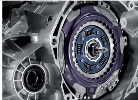
7-speed Double Clutch Transmission (DCT)
